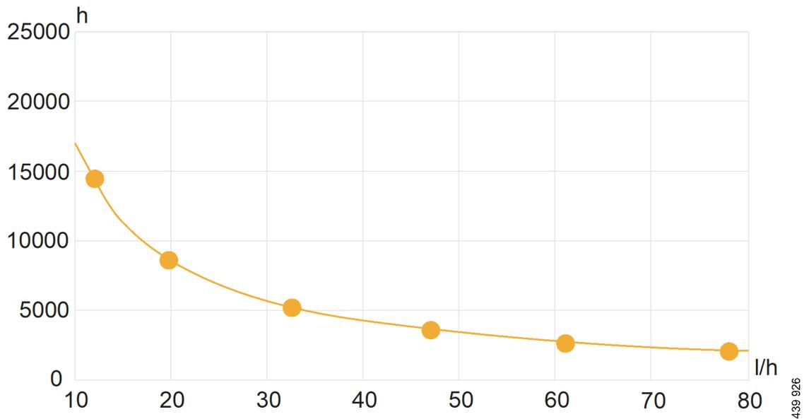
The graphs in the diagram show calculated driving time before particulate filter renewal.
