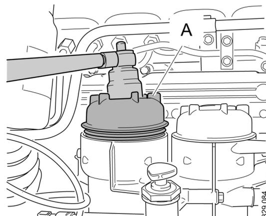
2. Unscrew the filter cover (A) and lift it up slowly with the filter element.
