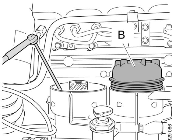
6. Unscrew the main filter cover (B) and lift it up slowly with the filter element.
