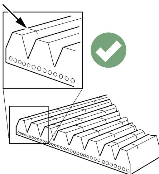
Example of a minor crack in the drive belt. The drive belt can be refitted.
