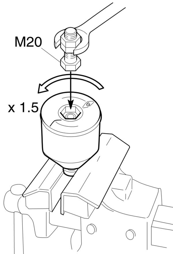
13. Remove the rotor cover by holding the rotor in both hands and tapping the rotor nut against the table. Never strike the rotor directly as this may damage its bearings.
