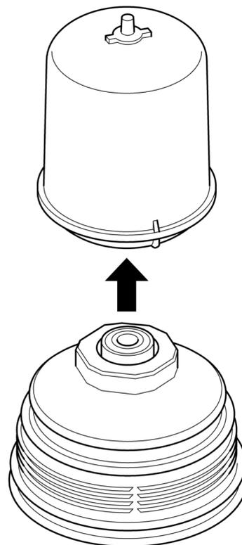
13. Press the rotor onto the cover.
