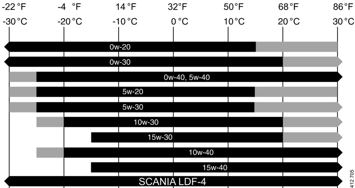
The illustration describes which ambient temperature in °C the viscosity class can handle for Scania-approved and market-approved oil grades. Note that the Scania-approved oil grades have a greater temperature range than market approved oil grades.
