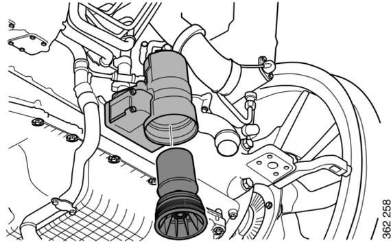
10. Remove the rotor by pulling it straight up from the cover. See illustration.
