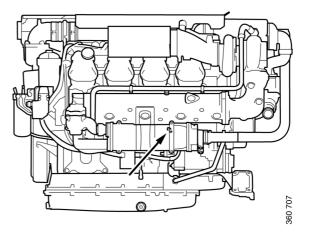
Drain nipple in the cylinder block (behind the heat exchanger).
