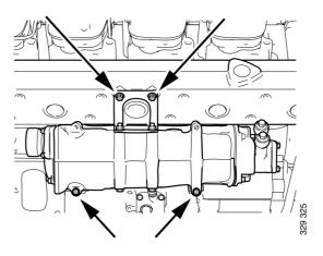
7. Remove the heat exchanger by holding it in the bracket, moving the heat exchanger slightly to the side and removing it.
