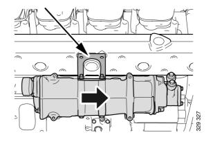
2. Fit all screws by hand and then tighten them. Tightening torque 50 Nm (37 lb/ft).
