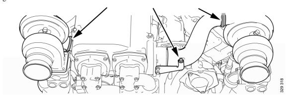
8. Remove the screws securing the charge air cooler.
