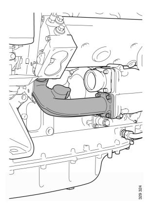
6. Remove the screws on the heat exchanger and the 2 upper screws on the exhaust manifold bracket.
