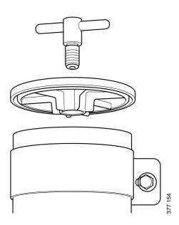
4. Remove the filter and fit the new filter.
