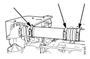
5. Remove all sea water pipes to and from the charge air cooler.
