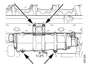
3. Lubricate and fit the coolant pipe from the heat exchanger. Angle the pipe from the thermostat housing inwards and push it onto the connection.
