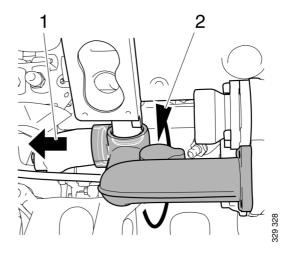
4. Fit the coolant pipe with the thermostat housing cover.
