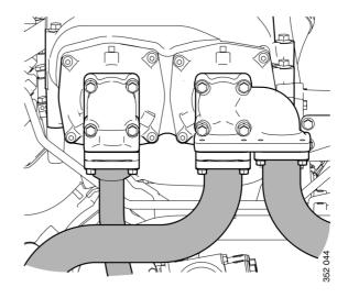
5. Fit the charge air pipe and the hose clamps.
