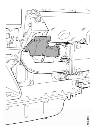
5. Remove the coolant pipe from the heat exchanger.
