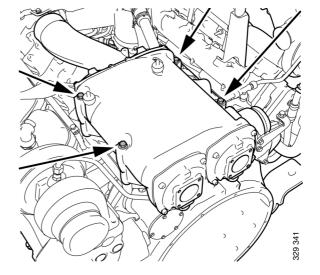
9. Lift out the charge air cooler.
