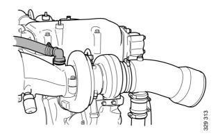
4. Loosen and remove the hose clamps for the charge air pipe.
